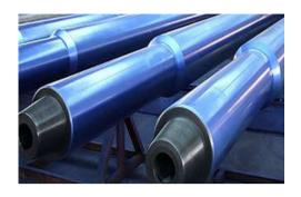
Drill collars are hollow, thick walled pipe with smaller nozzle, Per Unit Length of the drill collar is typically 4-5 times weight of the drill pipe. Drill collar are offered in all kinds, Round drill collar, spiral drill collar, non magnetic drill collar, square drill collar etc. We offer Drill collar in all variety of conventional and premium thread. Drill collars are available in R2 & R3 length.
