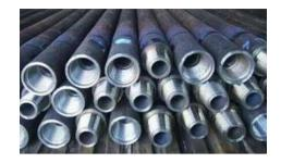
Drill pipe is hollow, thin walled, steel or aluminium alloy piping that is used on drilling rigs, it is hollow to allow drilling fluid to be pumped down the hole through the bit and back up through the annulus. It comes in a variety of sizes, strengths, and wall thicknesses, It is typically 27-32 feet in length(Range 2), Longer range in R3 up to 45 feet are also offered.
